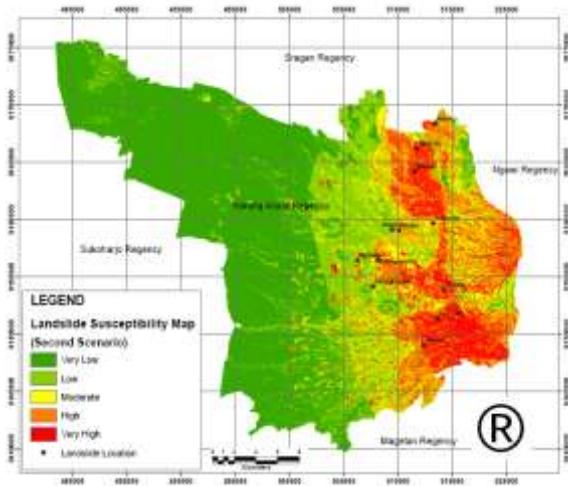
Fig. 2 Landslide susceptibility map of Karanganyar Regency, Central Java, Indonesia, developed in regional scale of 1:100,000 (Karnawati et al 2009 and 2011).
