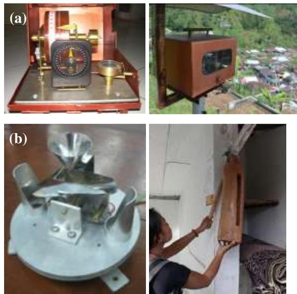
Figure 3. Early warning instruments consisting of (a) the extensometer and (b-left) the rain gauge, which also manually linked to the traditional “kentongan” (b-right).
