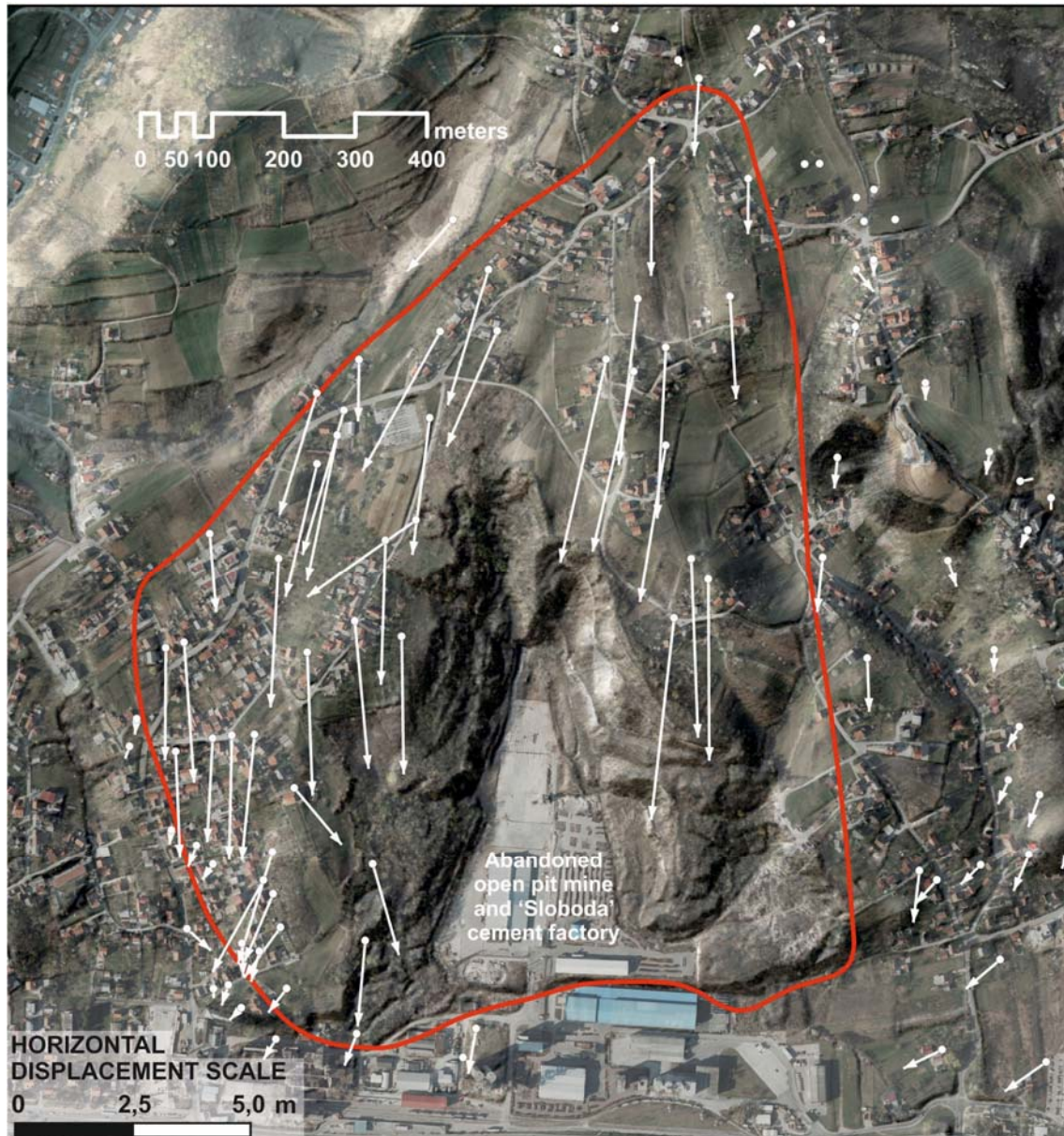
Fig. 1 Horizontal displacements (white arrows) at the Kostanjek landslide area in the period 1963-1988 based on interpretation of stereo pairs of aerial photographs from 1963, 1979, 1981, 1985 and 1988 (Ortolan and Pleško, 1992). Red line depicts the outline of the Kostanjek landslide according to interpretation by Ortolan (1996). In the background are maps from March 2012: hillshade map (with an azimuth of 315^\circ and a sun angle of 45^\circ ) generated from 2 \times 2 m bare earth DEM overlain by an orthophoto image. Devastated slopes of the abandoned open pit mine are clearly expressed by rough relief forms in the middle of the Kostanjek landslide. The former cement factory 'Sloboda' was placed in the plain area in the bottom middle part of the landslide.
