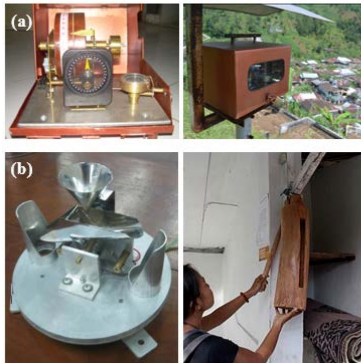
Fig. 3 Early warning instruments, consisting of (a-left and right) the extensometer and (b-left) the rain gauge, which also manually linked to the traditional “kentongan” (b-right)
