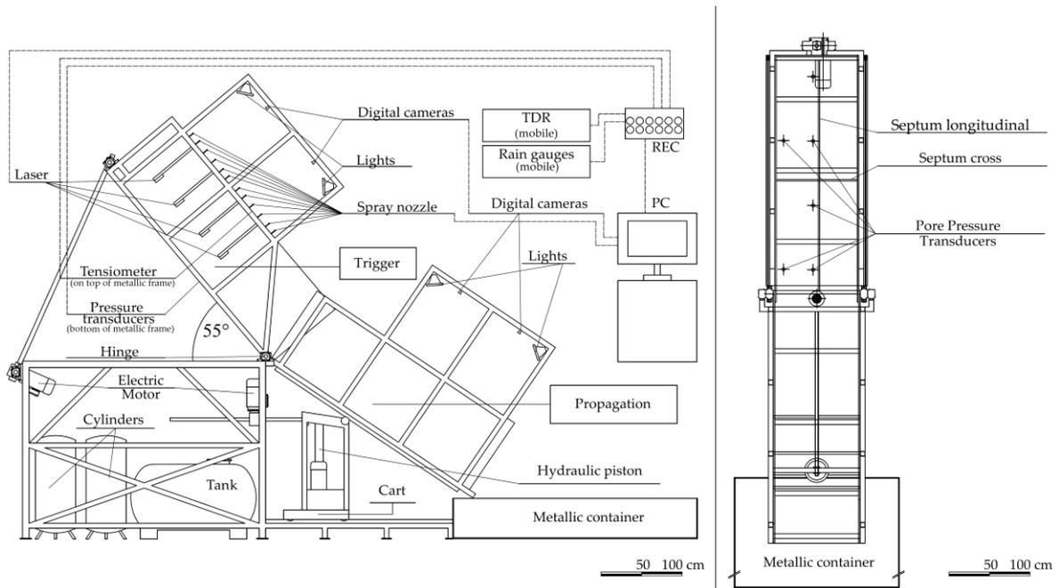
Figure 1. Section and plan of the mechanical components of flume.
